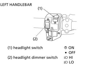
The headlight switch (1) is used to turn the headlights and assist headlight ON ( $\Re$ ) or OFF ( $\bullet$ ). The assist headlight turns on only when the dimmer switch (2) is in the HI ( $\equiv$ D) position. To operate, turn the switch to ON ( $\Re$ ) or OFF ( $\bullet$ ).
