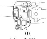
The engine stop switch (1) is used to stop the engine in an emergency. To operate, slide the switch to the OFF  $(\mbox{\ensuremath{\bowtie}})$  position. The switch must be in the RUN  $(\mbox{\ensuremath{\cap}})$  position to start the engine, and it should normally remain in the RUN  $(\mbox{\ensuremath{\cap}})$  position even when the engine is OFF.
