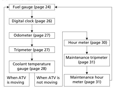
If there is a fuel warning with your ATV, the display will automatically change to the fuel gauge. If you try to change the display back to ordinary display, it will automatically return to the fuel gauge.
