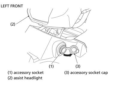
The accessory socket (1) is attached to the left side under the assist headlight (2). You can use the accessory socket to power a trouble light, spotlight, CB radio, or cell phone, etc.
