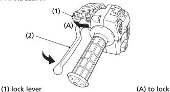
(2) rear brake lever/parking brake lever
