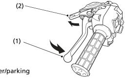
(1) rear brake lever/parking brake lever(2) P/R lever
