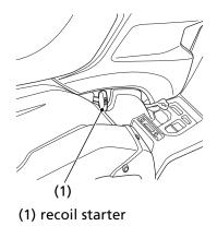
The recoil starter (1) is used to start the engine when the battery is low. See *Using the Recoil Starter (Canada only)* page 86.
