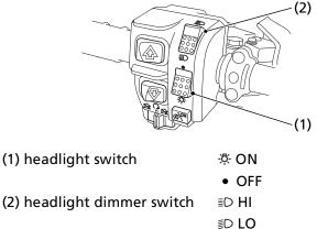
The headlight switch (1) is used to turn the headlights and assist headlight ON ( $\mathfrak{P}$ ) or OFF ( $\bullet$ ). To operate, turn the switch to ON ( $\mathfrak{P}$ ) or OFF ( $\bullet$ ).
