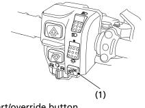
(1) start/override button औ<sup>®</sup> START or SPEED LIMITER OVERRIDE MODE
