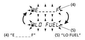
When the fuel gauge show " $E_{--}F$ " (4) and "LO FUEL" (5) blink 3 times alternately and fuel mark blinks, you should refuel as soon as possible.
