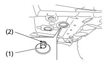
(1) engine oil drain bolt
