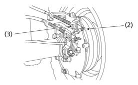
(2) brake lever adjusting nut(3) brake arm pin
