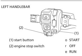
The start button (1) is used for starting the engine. Pushing the button in starts the engine. See *Starting Procedure*, page 71.
