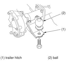
The trailer hitch (1) is located on the rear axle housing. To use the hitch, you'll need a proper size ball (2) as specified by the trailer manufacturer.
