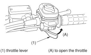
The throttle controls engine rpm (speed). To increase engine rpm, press the throttle lever (1) with your thumb. To reduce engine rpm, release pressure on the throttle lever. The throttle will automatically return to the closed position (engine idle) when you remove your thumb.
