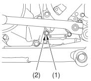
(1) transmission oil drain bolt (2) sealing washer
