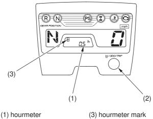
(2) hourmeter/odometer/ tripmeter select button
