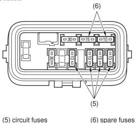
6. To check or replace a circuit fuse (5), pull the old fuse out of its retaining clips.
