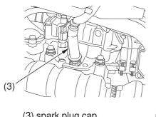
(3) spark plug cap(4) center electrode
