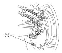
(1) rear brake drain bolt
