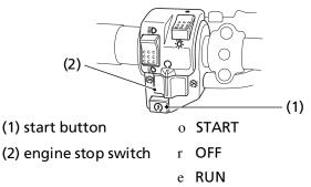
The start button (1) is used for starting the engine. Pushing the button in starts the engine. See *Starting Procedure*, page 72.
