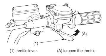
The throttle controls engine rpm (speed). To increase engine rpm, press the throttle lever (1) with your thumb. To reduce engine rpm, release pressure on the throttle lever. The throttle will automatically return to the closed position (engine idle) when you remove your thumb.
