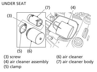
11. Install the air cleaner on the air cleaner body.
