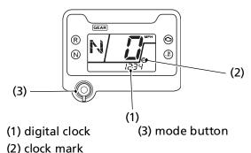
After the battery is reconnected (page 183), check the clock. Readjust the clock if necessary.
