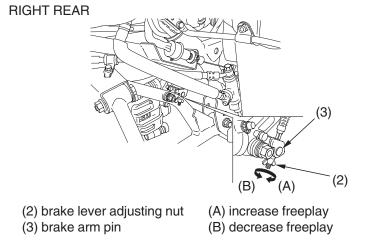
Adjust the freeplay of the rear brake lever/parking brake lever with the front wheels pointed straight ahead.
