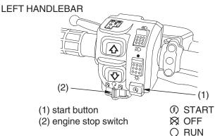
The start button (1) is used for starting the engine. Pushing the button in starts the engine. See Starting Procedure, page 64.
