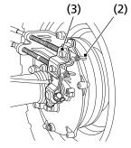
(2) brake lever adjusting nut(3) brake arm pin
