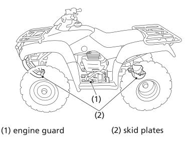
The engine guard (1) protects the engine crankcase.
