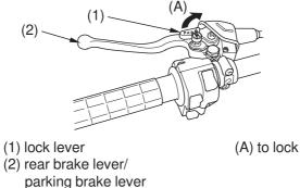
The lock lever (1) on the rear brake lever/parking brake lever (2) allows it to be used as a parking brake. To operate, first squeeze the rear brake lever/parking brake lever using your left hand and then lock it with the lock lever using your right hand. See *Parking* page 72.
