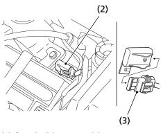
(2) fuse holder assembly(3) fuse holder
