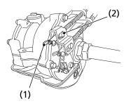
(1) brake lever adjusting nut
