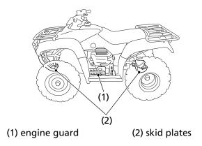
The engine guard (1) protects the engine crankcase. The skid plates (2) protect the frame and rear final gear case. Check the guard and plates for cracks, damage or looseness at intervals shown in the Maintenance Schedule.
