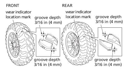
To check the condition of a tire tread, measure the groove depth in the center of the tire, or check the wear indicator.
