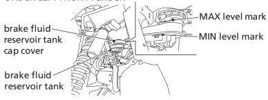
It should be between the MIN and MAX level marks. If the level is at or below the MIN level mark, check the brake pads for wear (page 189).
