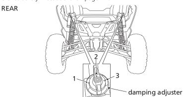
The damping adjuster has 3 positions for different load or driving conditions.
