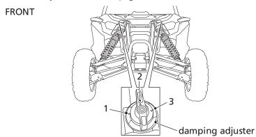
The damping adjuster has 3 positions for different load or driving conditions.
