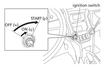
To stop the engine, turn the ignition switch to the OFF (w) position. Remember to shift into the park (P) position and remove the key if you plan to leave the vehicle.
