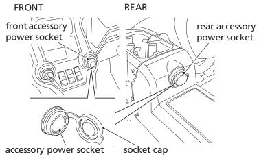
To use an accessory power socket, the engine must be running.
