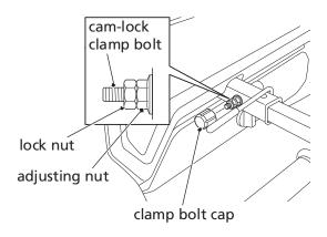
Do not apply a grease or lubrication to the handhold slider surface and cam-lock clamp.
