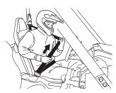
To unlatch a seat belt, press the red PUSH button on the buckle.
