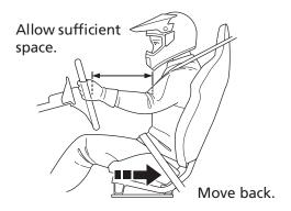
Always make driver seat adjustment before driving. The passenger seats do not have seat position adjustments.
