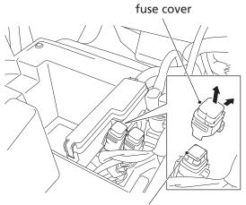
brake traction control system (BTCS) fuse
