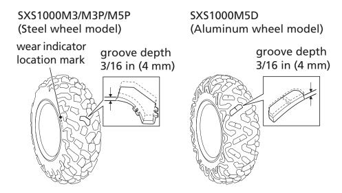
To check the condition of a tire tread, measure the groove depth in the center of the tire, or check the wear indicator. For best performance, you should replace a tire before the tread depth at the center reaches the following limits:
