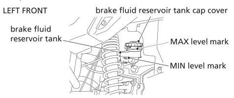
It should be between the MIN and MAX level marks. If the level is at or below the MIN level mark, check the brake pads for wear (page 184).
