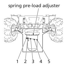
The spring pre-load adjuster has 5 positions for different load or riding conditions. Before adjusting the spring pre-load, jack up your Honda SXS (page 132) to avoid damaging the adjusters.
