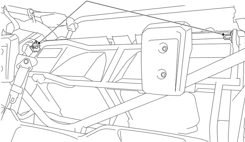
Lubricate the front seat latch as shown in the following illustration.
