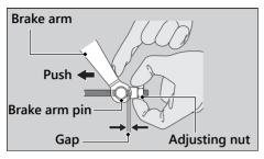
After adjustment, confirm the freeplay of the brake lever.
