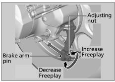
Apply the brake several times and check for free wheel rotation after the brake lever is released.
