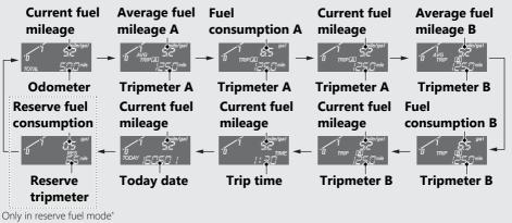
\* Reserve fuel mode: When the 1st (E) segment of the fuel gauge flashes, the reserve tripmeter display and reserve fuel consumption display can be selected.
