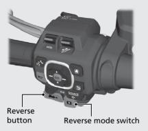
When you are ready to back up, press and hold the Reverse button. The vehicle will move in reverse as long as you hold the button down. ("R" is displayed on the gear position indicator.)
